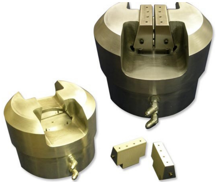
Grip components (below) and wedge grip assembly (above)
